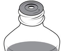
Liquid medication bottle with press-in oral syringe adapter
